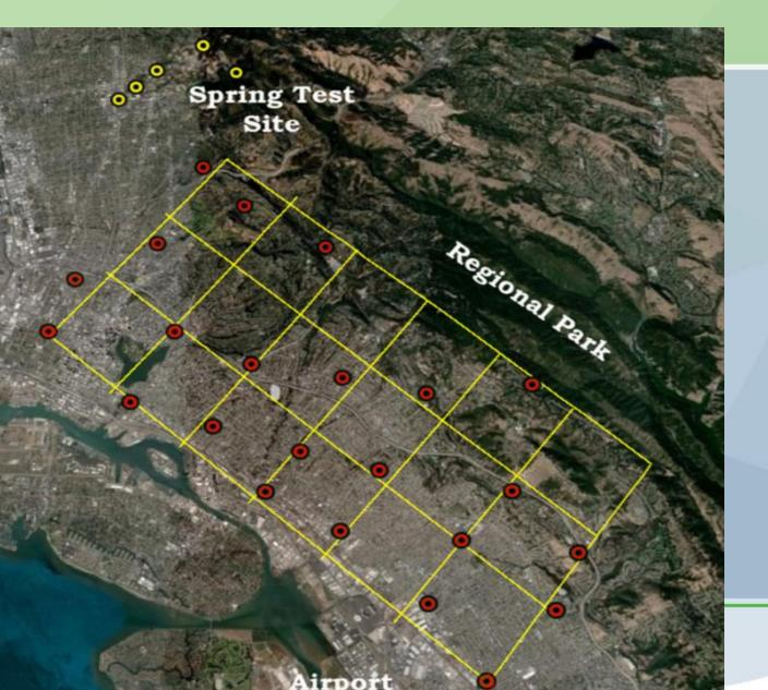
A 36 node, dense network is being deployed currently. Each node includes measurements of CO<sub>2</sub>, NO<sub>2</sub>, CO, O<sub>3</sub>, P, T, RH. Rough spacing between nodes is 2km over 27 sq. miles.
